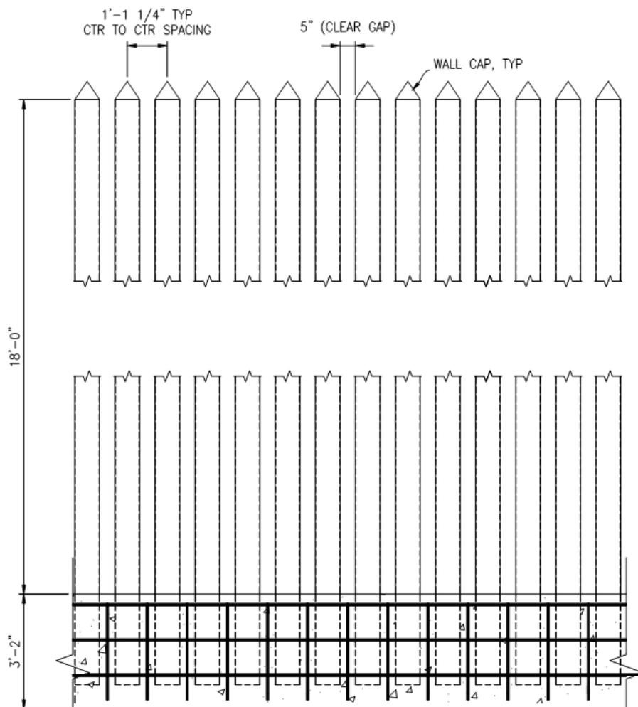
Figure 6.2. TGR typical wall elevation
