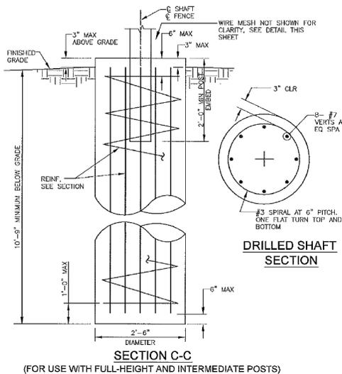
Figure 5.5. Typical K-2A fence foundation detail (RJM Architecture 2010)
