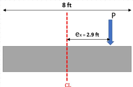
When Eccentricity exceeds the Kern, the pressure distribution under the footing takes a triangular shape as shown in the figure below. For this type of situation, the pressure Qmax becomes equal to 2P/3C.
