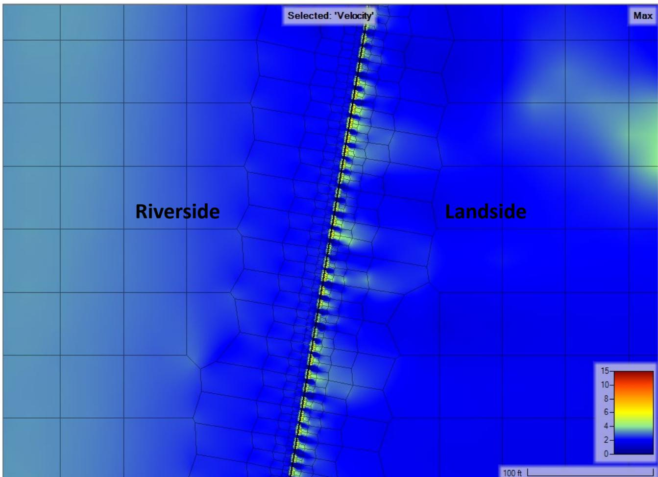
Figure 4.30. Maximum velocity plumes along western portion of fence
