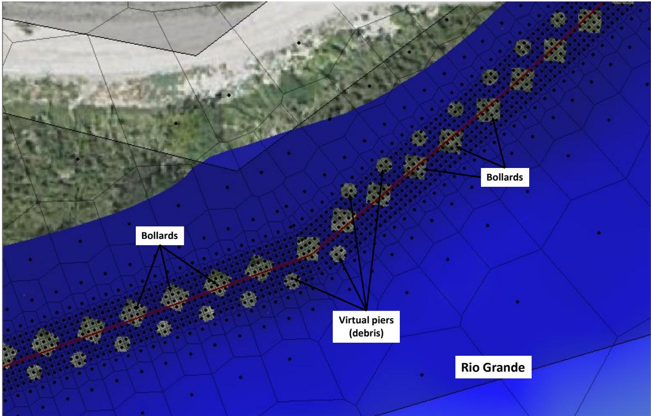
Figure 4.2. TGR bollard fence and virtual pier terrain (enlarged)
