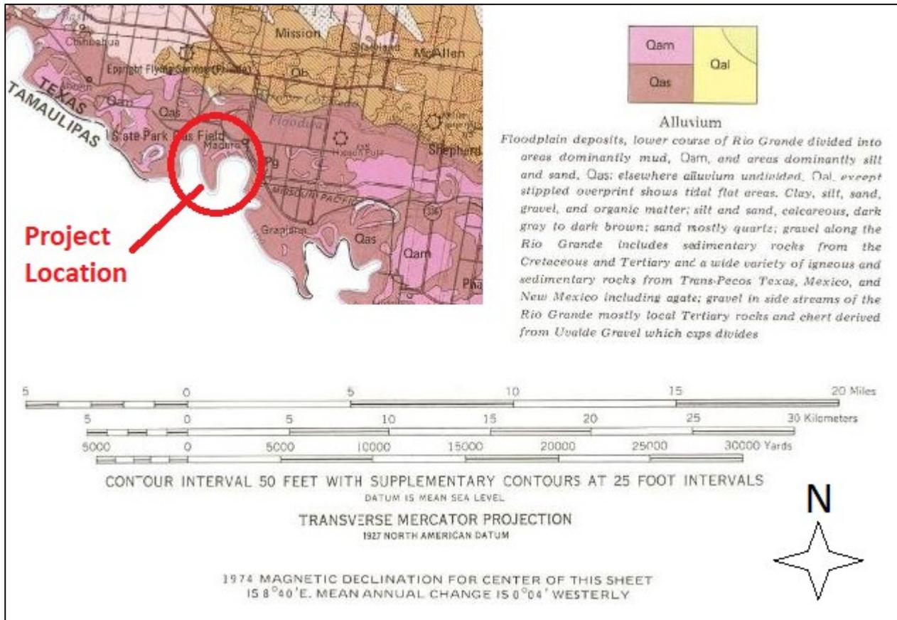
Figure 5.1. Geologic map showing surficial soils at and near the project location (modified from Barnes et al. 1976)
