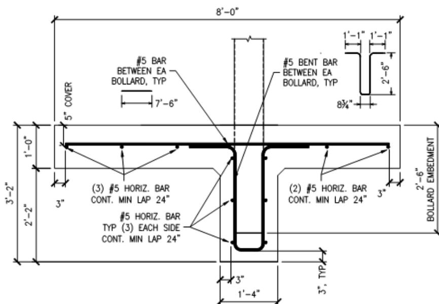
Figure 6.5. TGR typical reinforcement section
