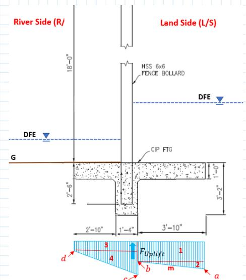
Uplift Pressure Below Shear Key:
