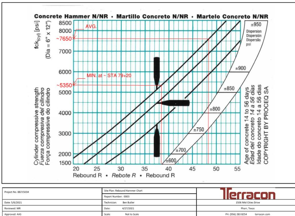
Figure 6.10. Rebound hammer converting chart
