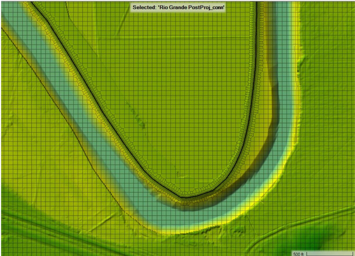
Figure 4.14. Arcadis 2D area post-project partial computational mesh
