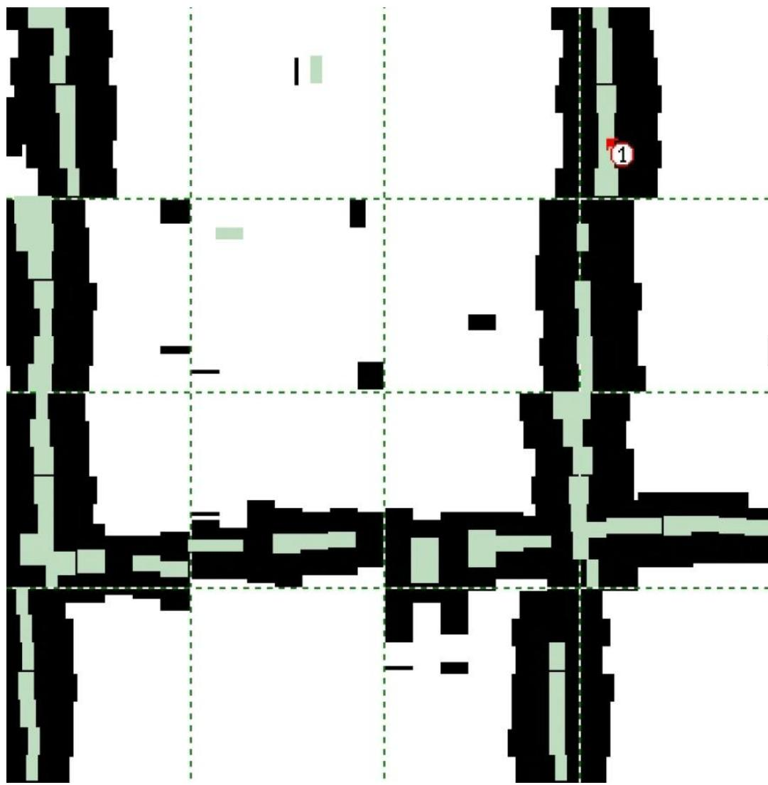
Marker 1: Bar size verified to be #5 bar by Ferroskan
