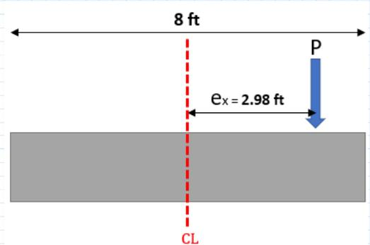
When Eccentricity exceeds the Kern, the pressure distribution under the footing takes a triangular shape as shown in the figure below. For this type of situation, the pressure Q<sub>max</sub> becomes equal to 2P/3C. Here, P is total vertical force, and C is resultant location.
