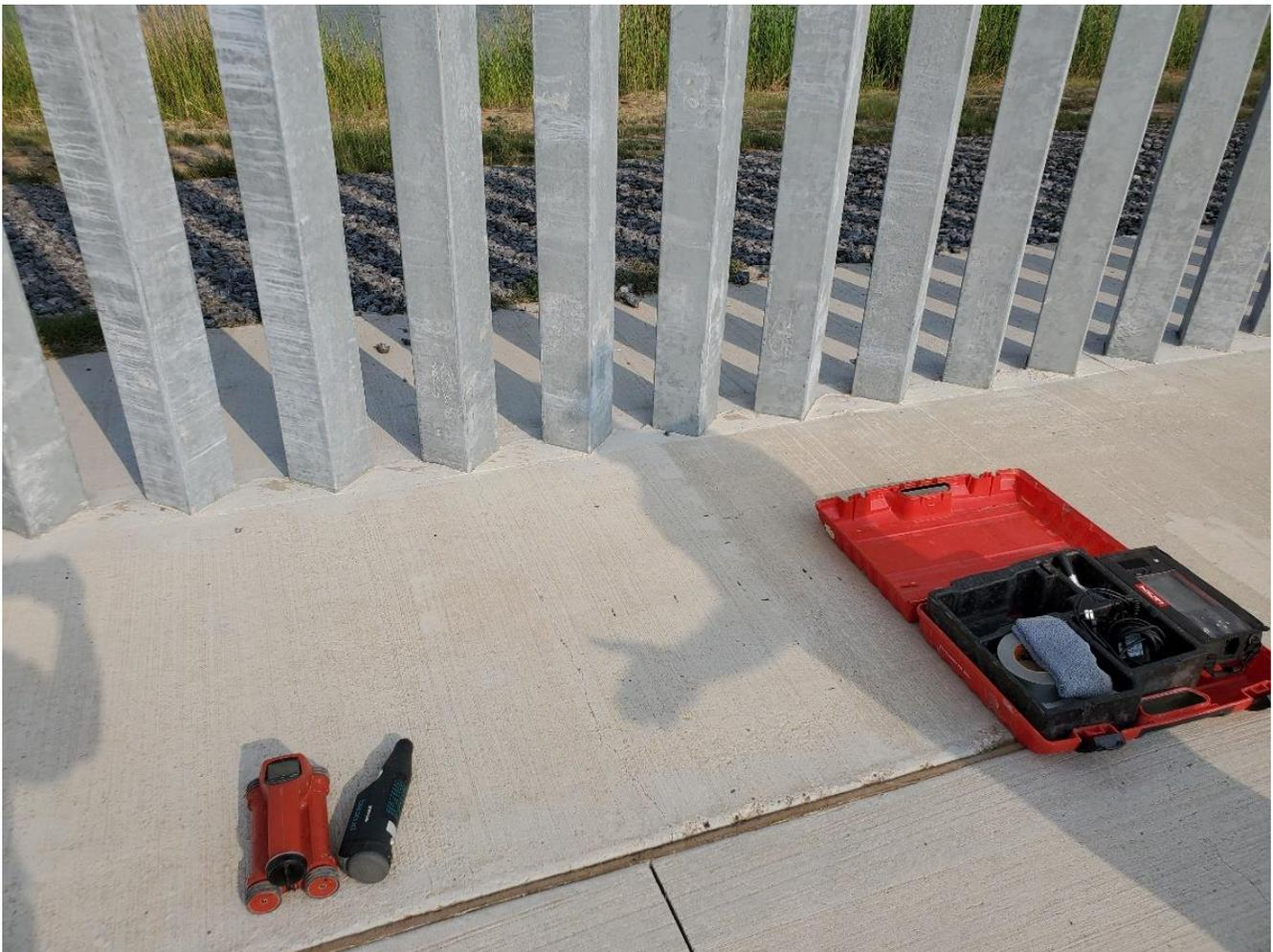
Figure 16: Typical GPR Test Location for Rebar Spacing and Concrete Strength
