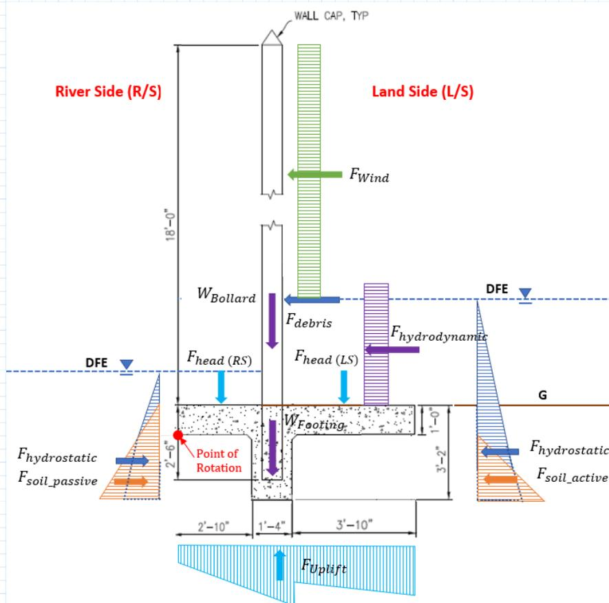
*Loading Diagram of Typical Bollard Fence for Case C (Rising Waters from Land Side)*
