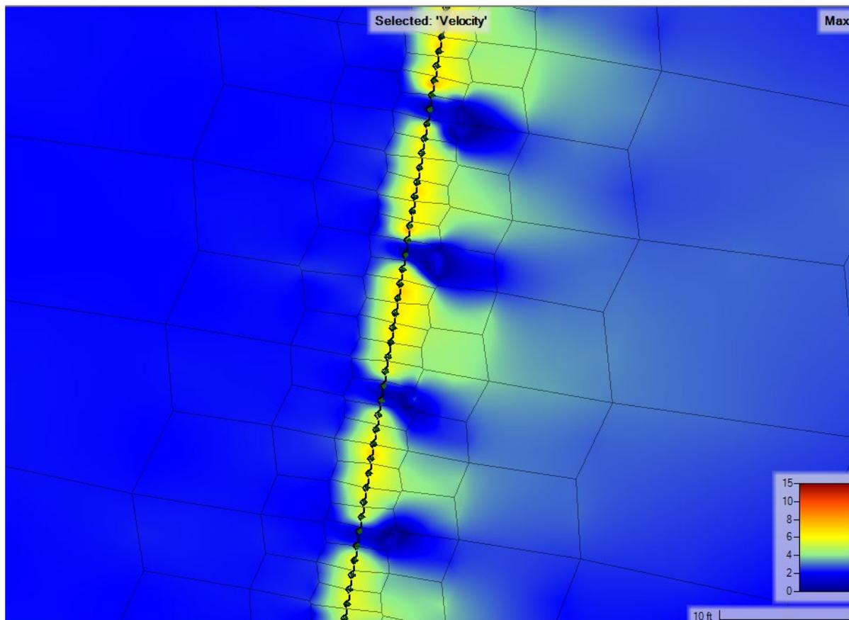
Figure 6.11. Maximum velocity plumes through typical unblocked openings on western portion of fence
