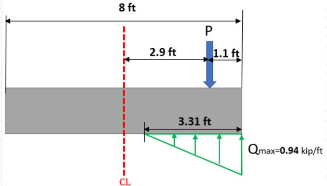
However, from equilibrium of forces, the area of the pressure triangle has to be equal to the resultant vertical force. Therefore,  $P = 0.5 \cdot B \cdot Q_{max}$ .
