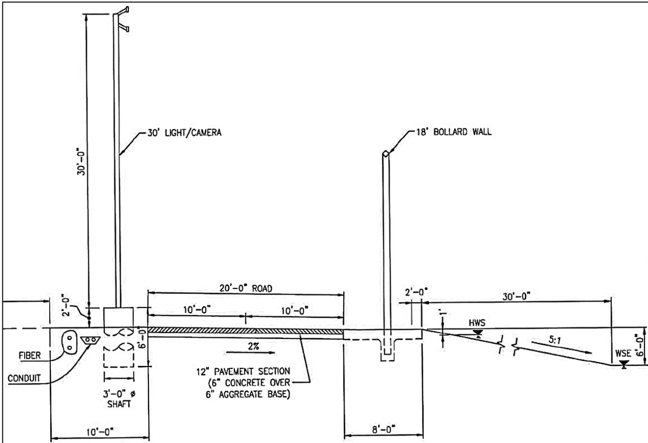
Figure 6: Typical Fence Section with Road and Utility Poles from Plans by TGR Dated October 30, 2019
