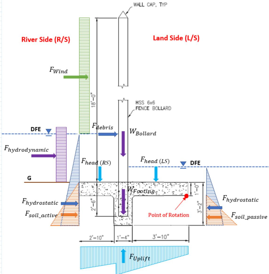
*Loading Diagram of Typical Bollard Fence for Case A and B (Rising Waters from River Side)*
