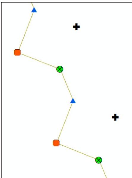
Figure 4.10. Breaklines created from upstream, downstream, and river side points
