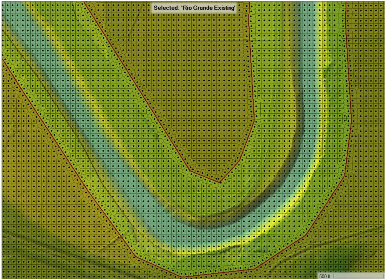
Figure 4.13. Arcadis 2D area pre-project partial computational mesh
