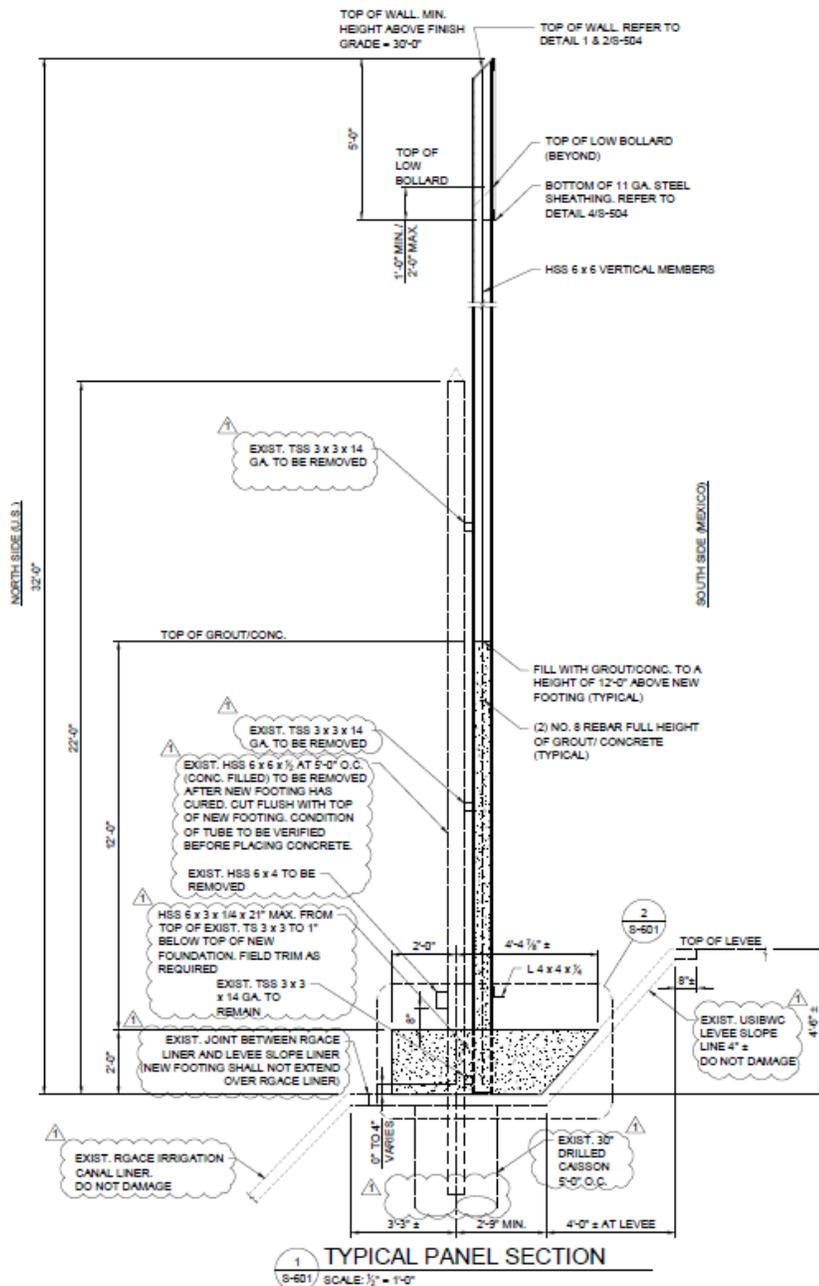
Figure 5.6. Fence foundation for Segment D-3, El Paso, TX (Benham 2020)
