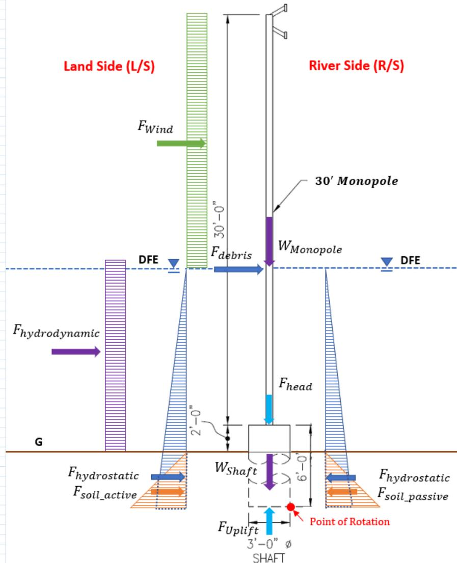
*Loading Diagram of Typical Monopole for Case C
