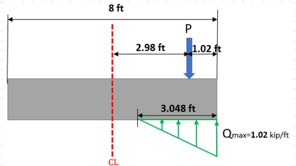
Length of the Pressure Triangle  $B := \frac{P_{down}}{0.5 \cdot Q_{max}} = 3.048 \text{ ft}$
