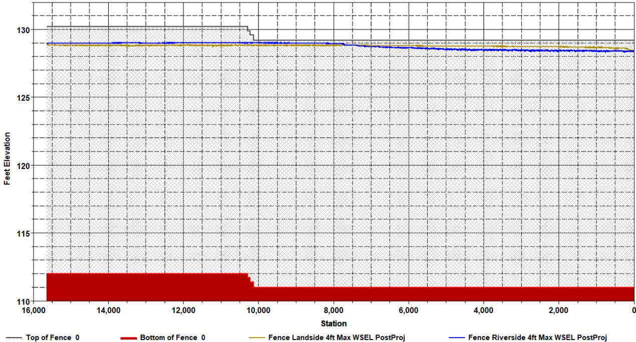
Figure 4.33. Profile showing fence base (dark red), top of bollards (gray), and maximum water surface elevations on land (orange) and river (blue) sides of fence
