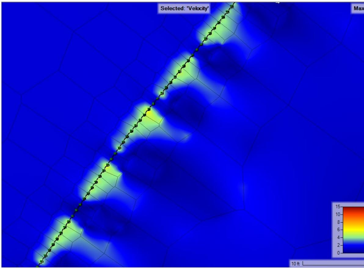
Figure 6.12. Maximum velocity plumes through typical unblocked openings on eastern portion of fence
