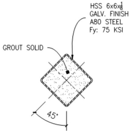
Figure 6.3. TGR typical bollard section
