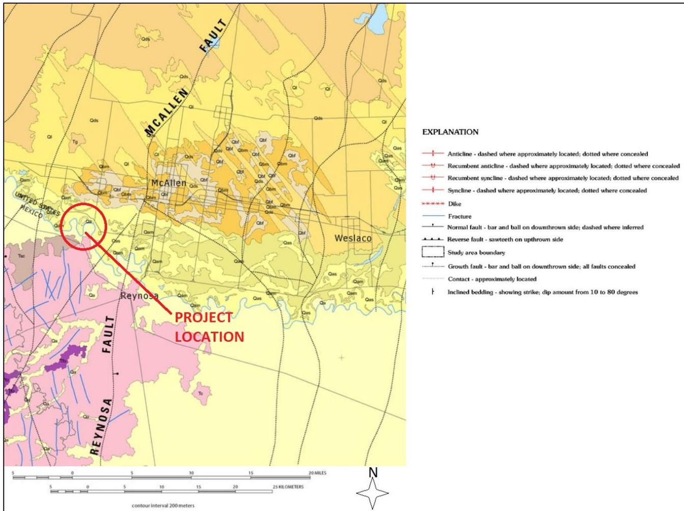
Figure 5.2. Faults near the project area (modified from Page et al. 2005)
