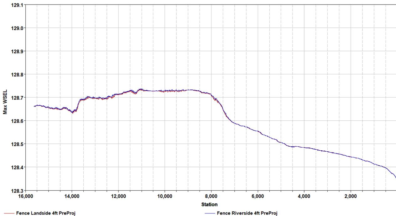
Figure 4.18. Pre-project peak water surface elevation profiles on land (red line) and river (blue line) sides of fence line
