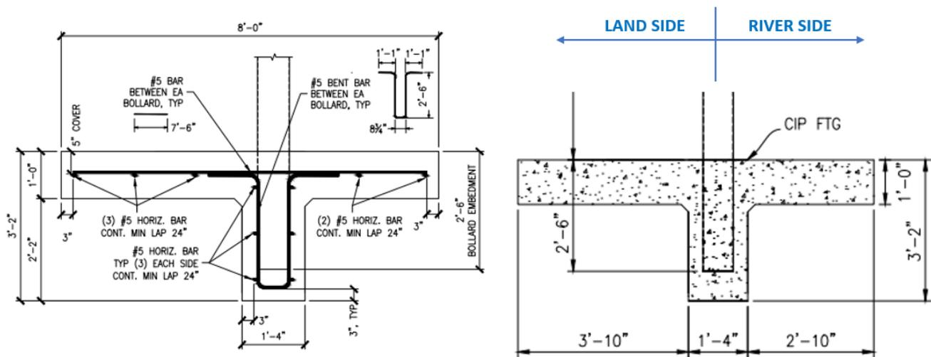
Figure 5.4. Sections of the fence foundation (Fisher 2019)
