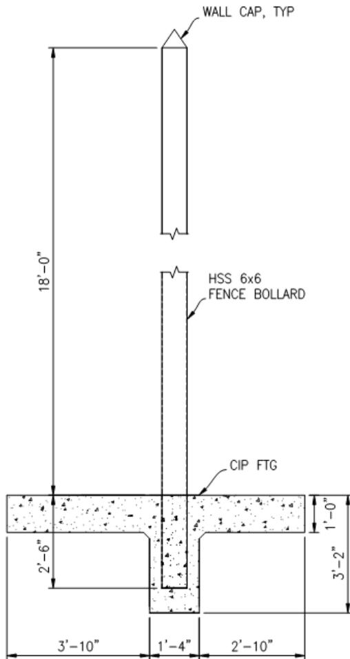
Figure 6.4. TGR typical bollard fence section
