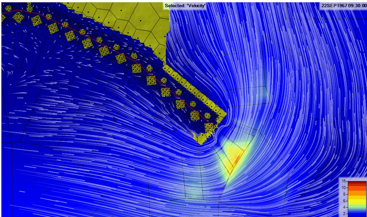
Figure 4.5. TGR HEC-RAS model-simulated velocity at downstream fence terminus
