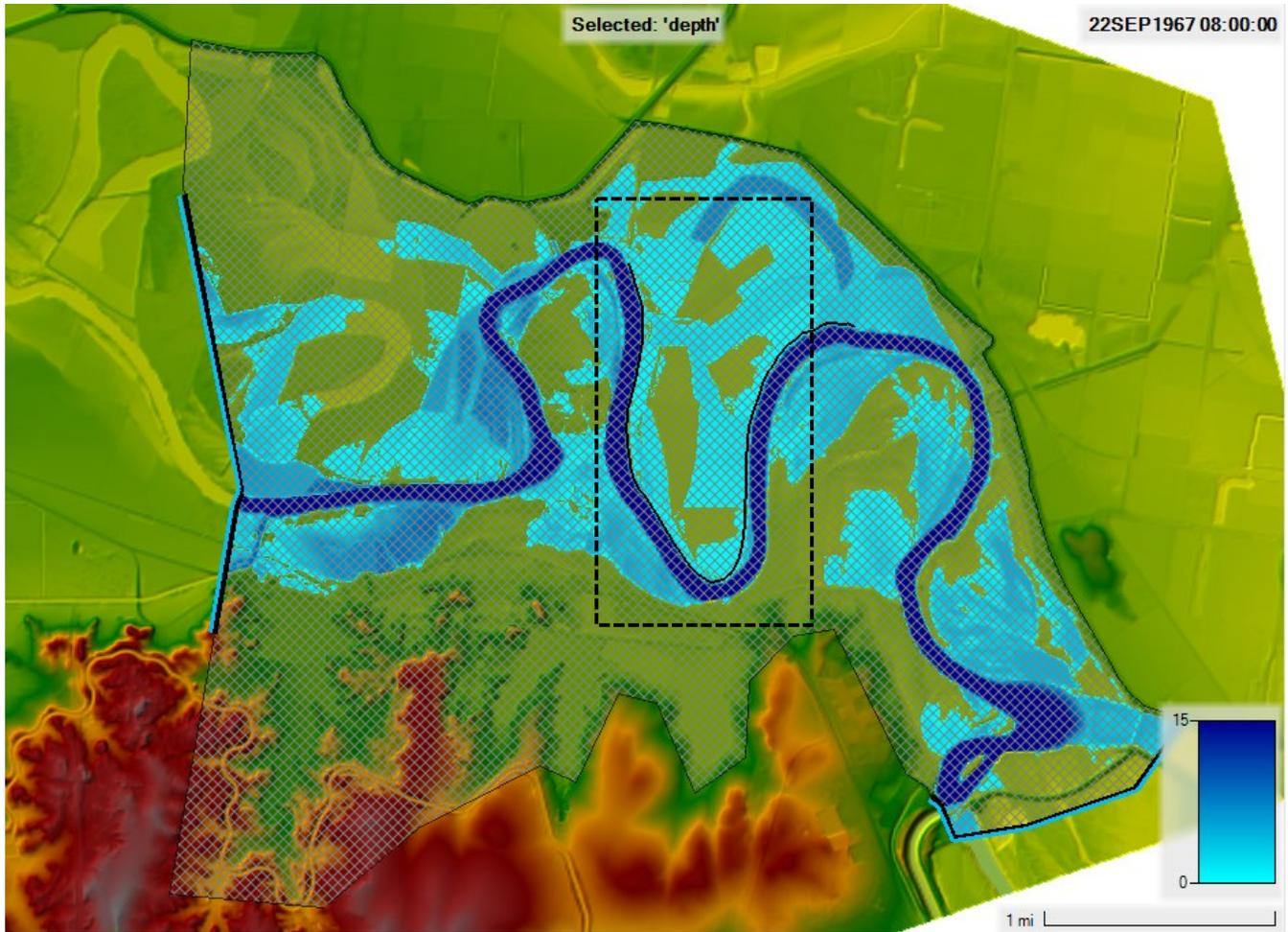
Figure 4.15. Pre-project depth of inundation (September 22, 1967, 08:00)
