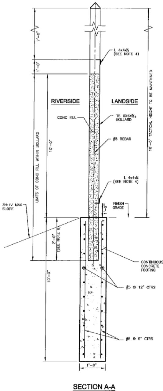
Figure 5.7. Fence foundation for Segment O-4 B, Mission Levee (L&G 2009)
