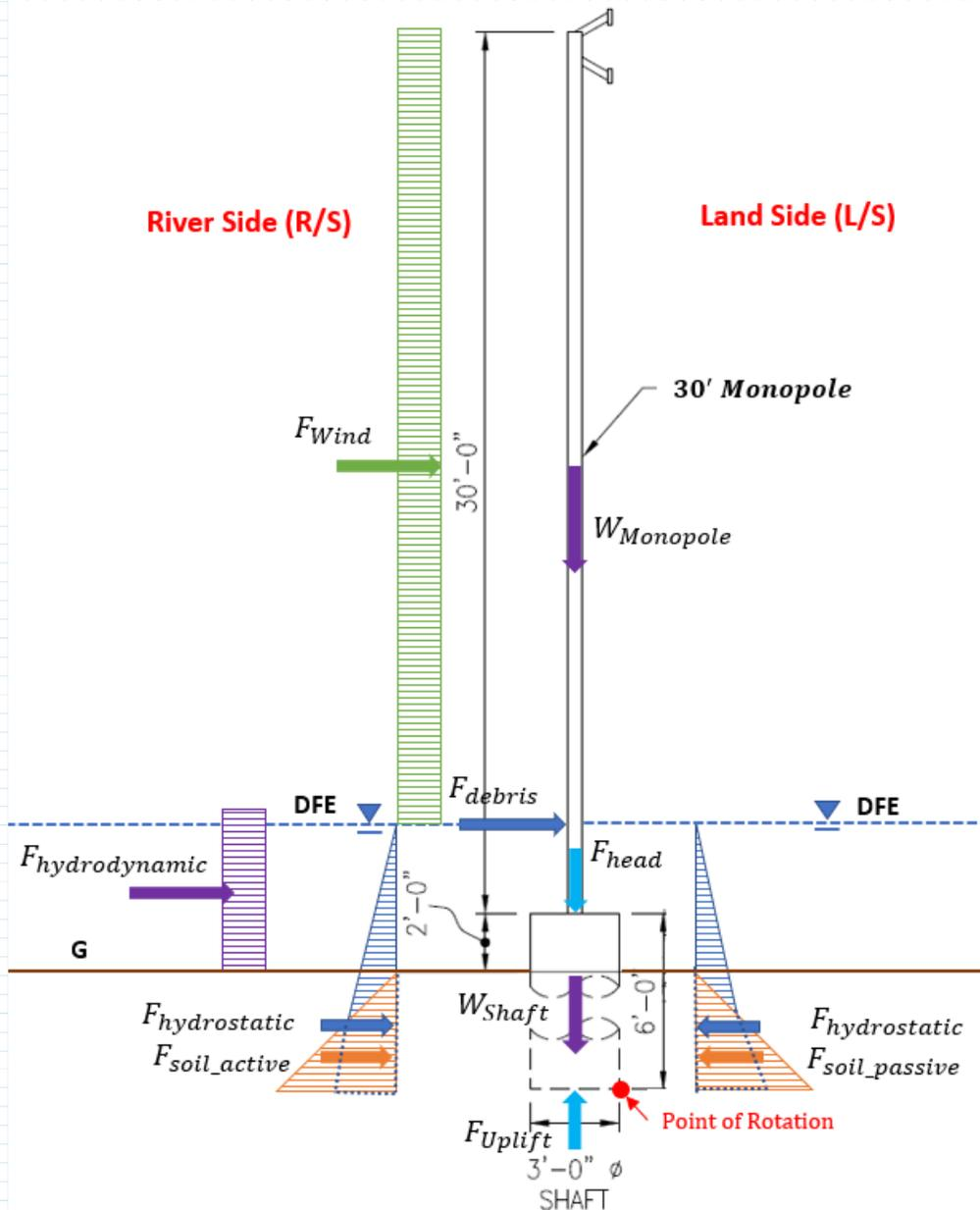
Loading Diagram of Typical Monopole for Case A (Rising Waters from River Side)
