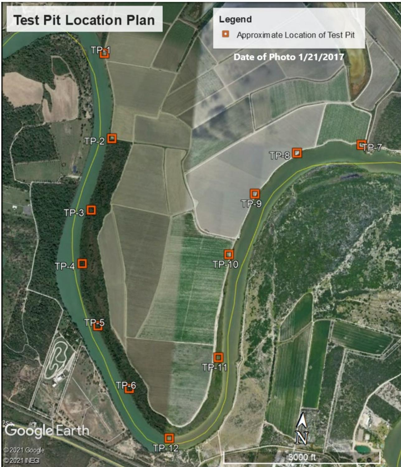
Figure 5.3. Approximate location of test pits excavated during site investigation in April 2021
