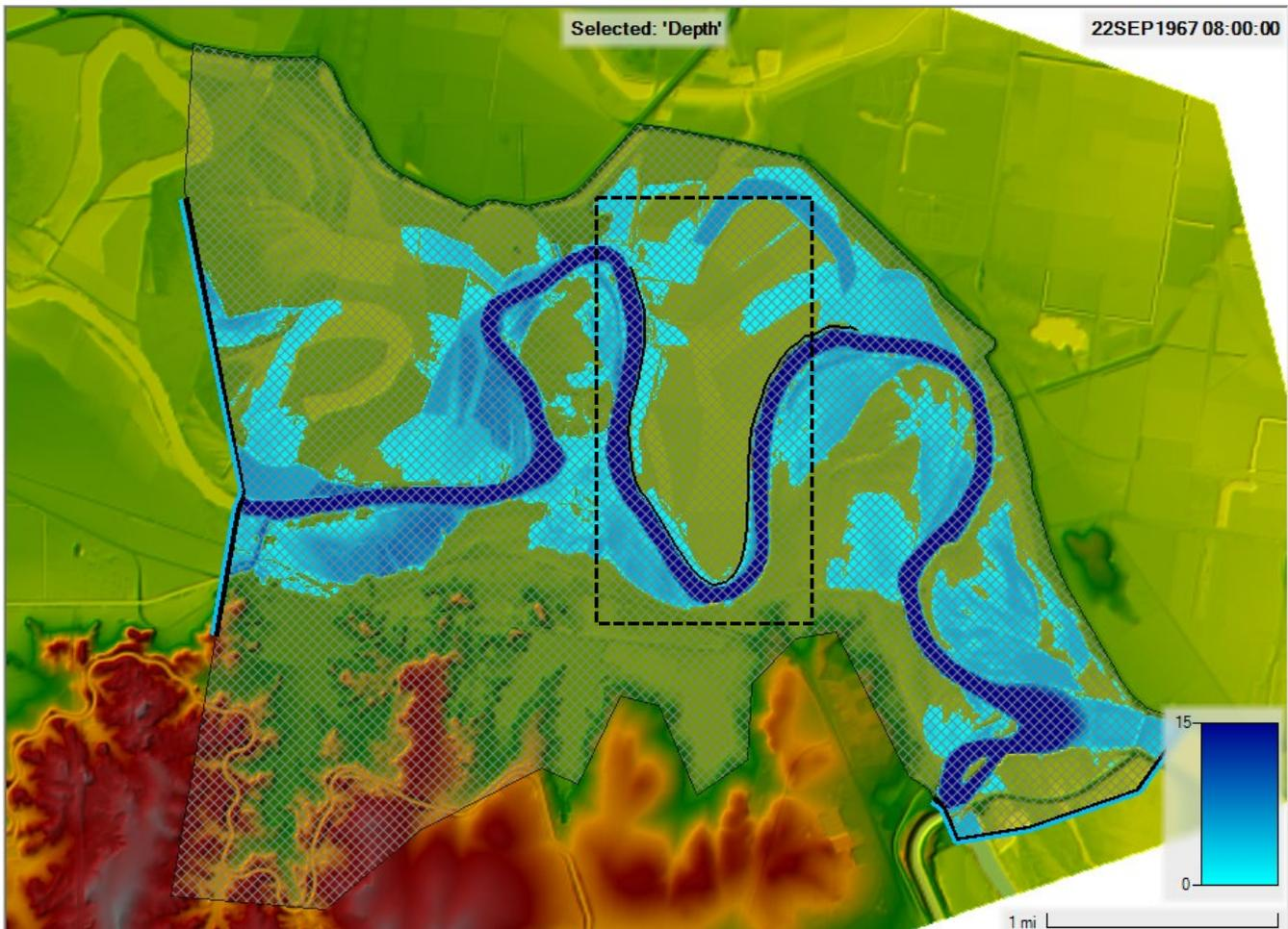
Figure 4.16. Post-project depth of inundation (September 22, 1967, 08:00)
