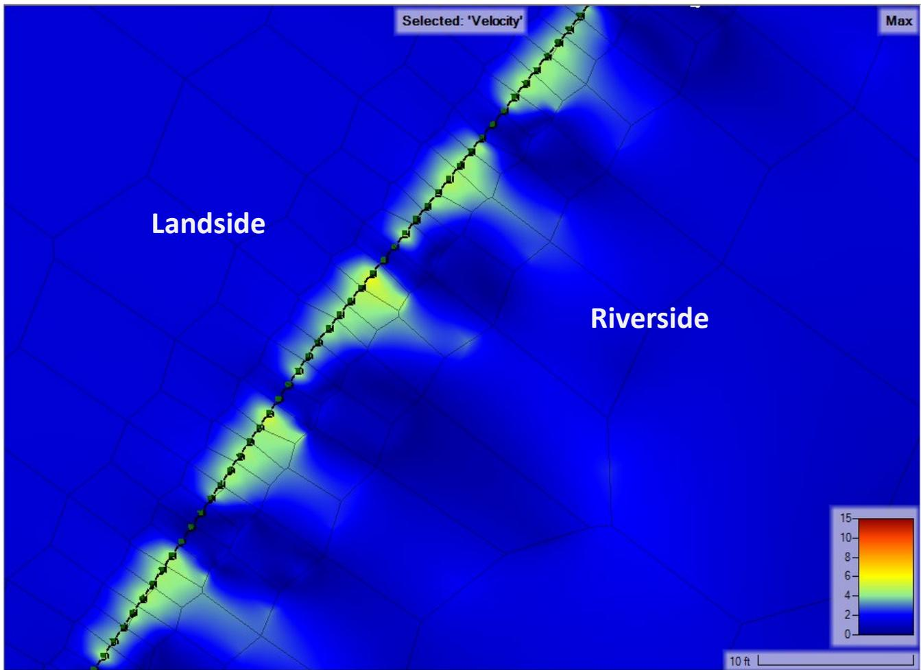
Figure 4.31. Maximum velocity plumes through typical unblocked openings on eastern portion of fence
