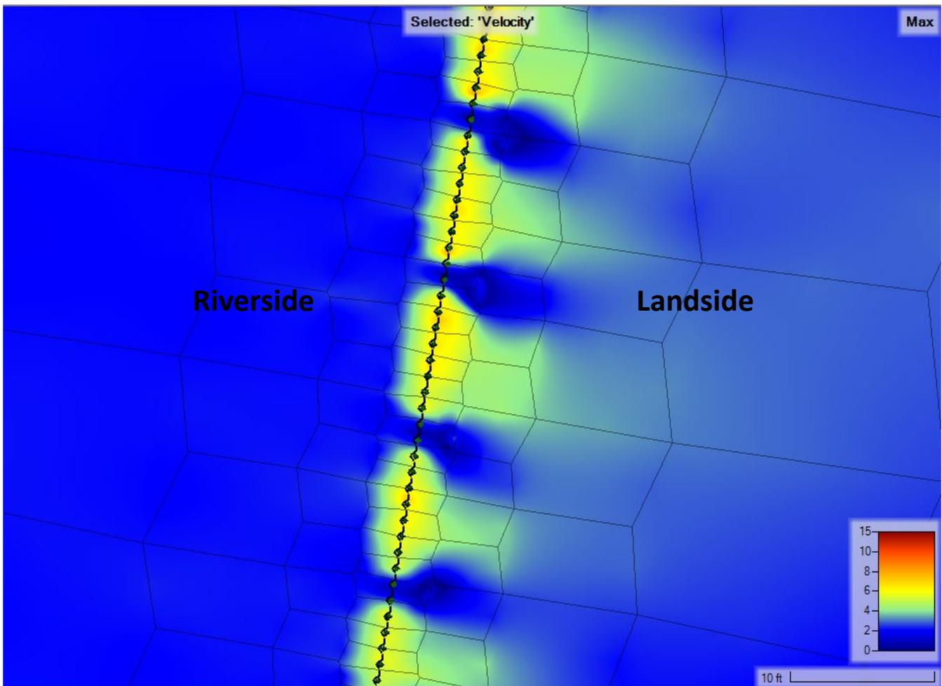
Figure 4.29. Maximum velocity plumes through typical unblocked openings on western portion of fence
