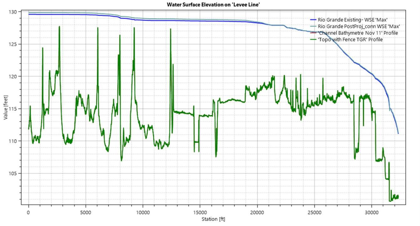
Figure 4.28. Maximum water surface elevation along Mission Levee (light blue – post-project, blue – pre-project, green – base elevation)
