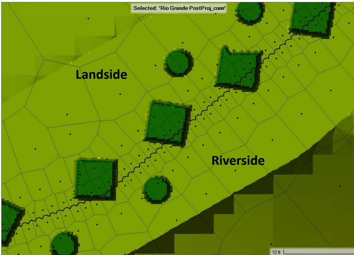
Figure 4.7. Sample TGR model fence terrain with blockage by piers
