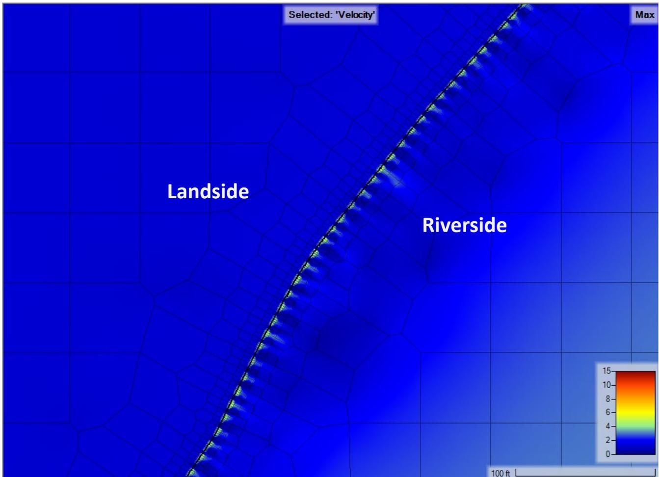
Figure 4.32. Maximum velocity plumes along eastern portion of fence
