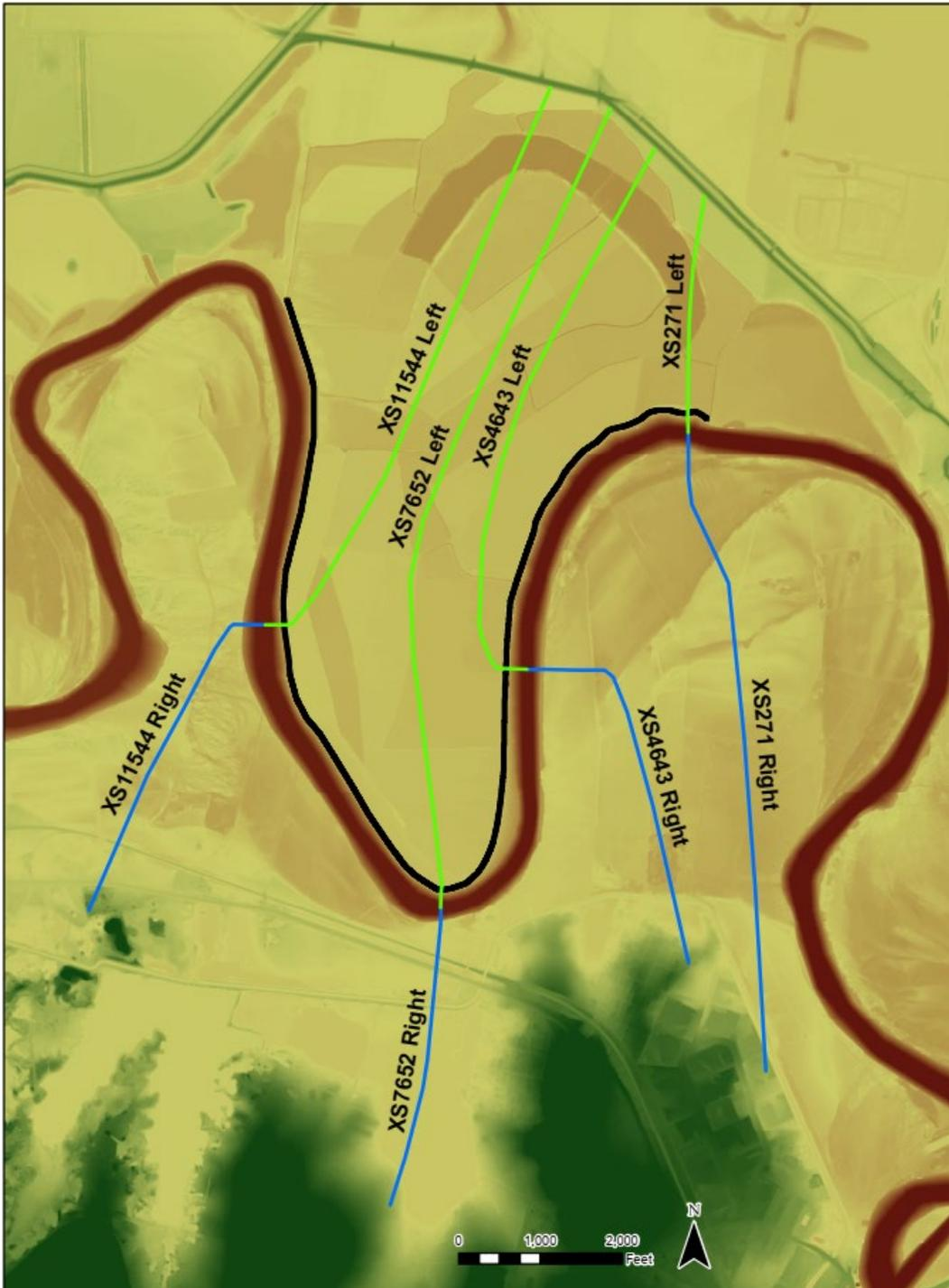
Figure 4.27. Profile lines for which changes in maximum water surface elevations and maximum flows were derived for use as IBWC-designated flow deflection indicators
