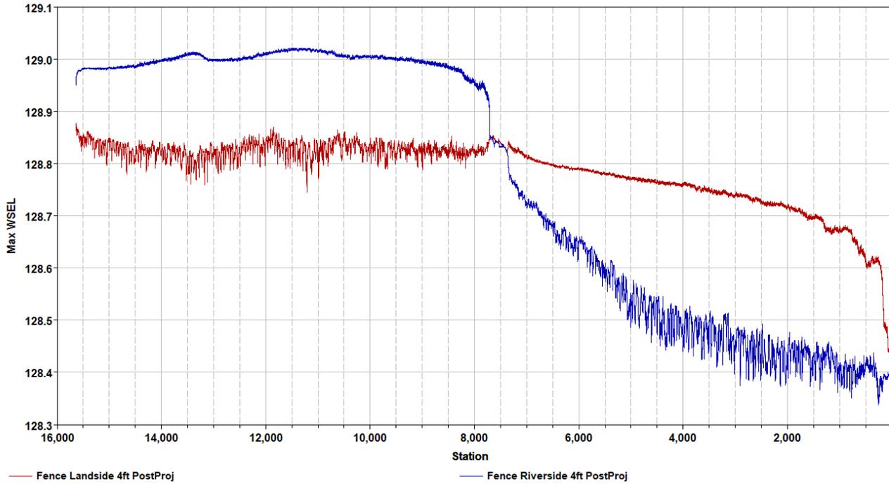
Figure 4.17. Post-project peak water surface elevation profiles on land (red line) and river (blue line) sides of fence
