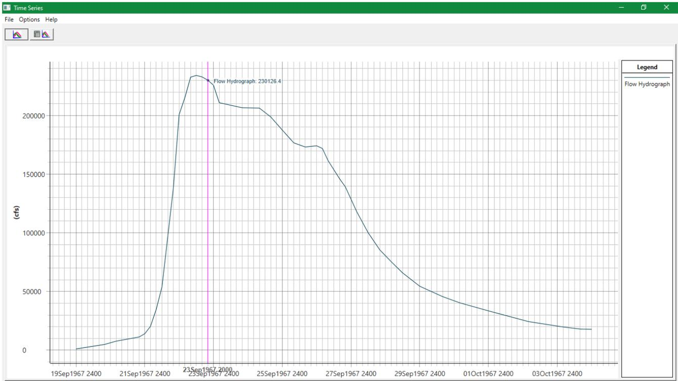
Figure 4.3. TGR HEC-RAS model discharge hydrograph upstream boundary condition
