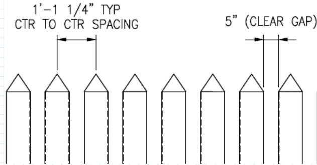
*Bollard Fence Elevation
