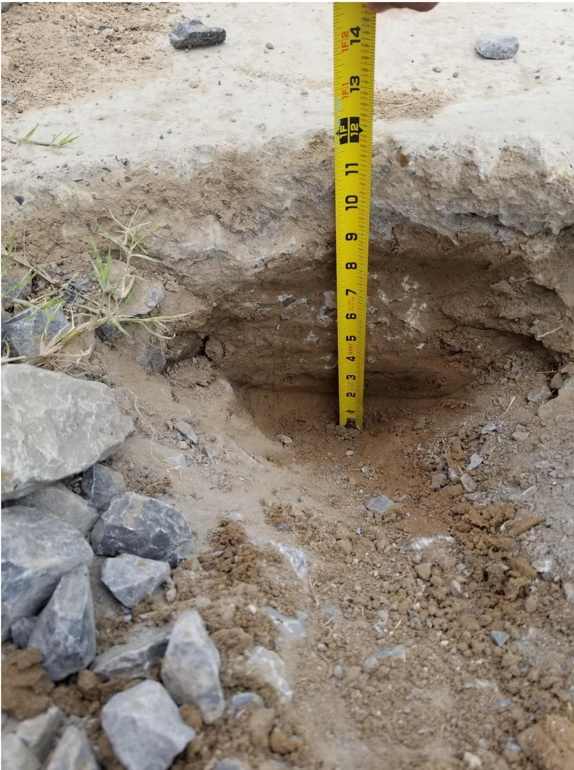
Figure 15: Footing Depth Measurement of Riverside Edge Near STA 156+00
