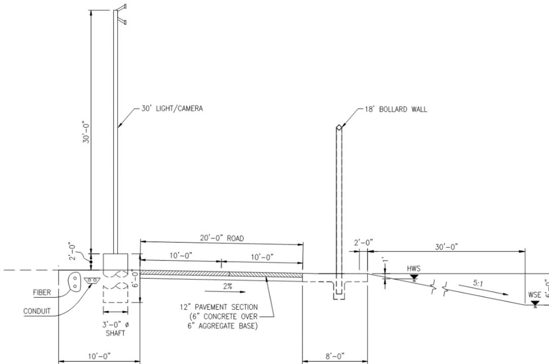
Figure 6.1. TGR typical system cross section
